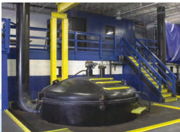
Vacuum furnace with a hot zone of 51" diameter x 80" depth.
