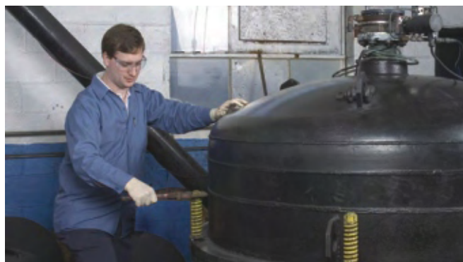
Vacuum furnace with a hot zone of 28" diameter x 50" depth
