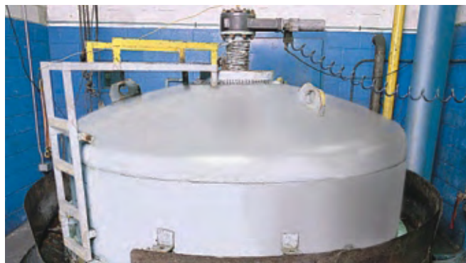
Vacuum furnace with a hot zone of 40" diameter x 80" depth.
